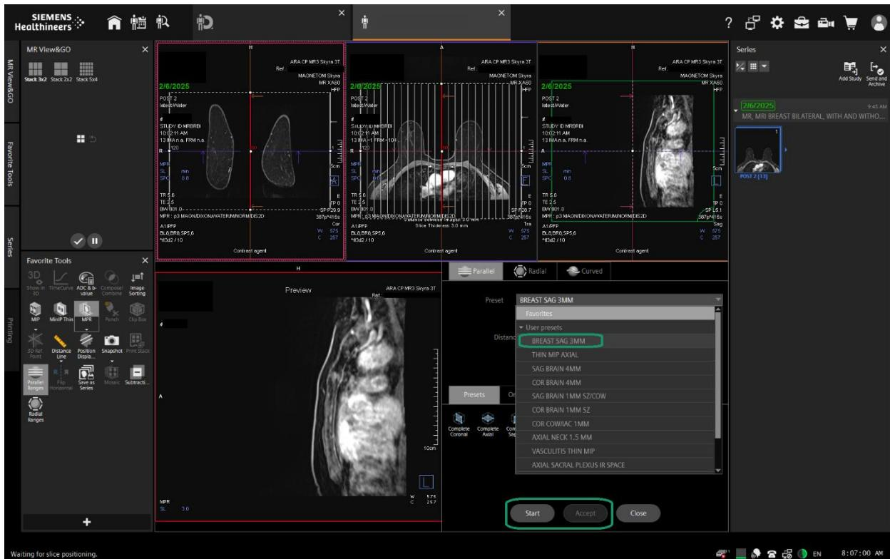
To create the **TIME MIP**, load each post sub dynamic into **View&GO** (POST 1\_W\_SUB, POST 2\_W\_SUB, POST 3\_W\_SUB, POST 4\_W\_SUB, and POST 5\_W\_SUB)
